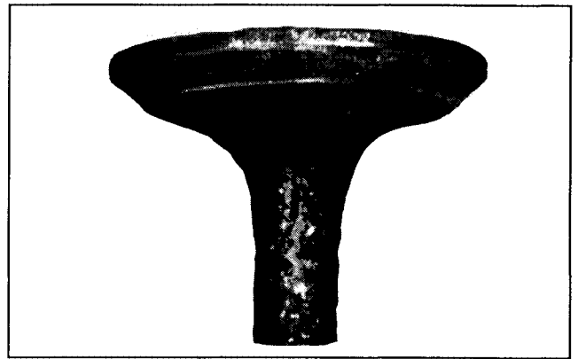
Stem Corrosion: Moisture from the fuel or from condensation are the most common causes of valve stem corrosion. Condensation occurs from improper preservation during storage and when engine is repeatedly stopped before it has a chance to reach normal operating temperatures. Replace corroded valves.
