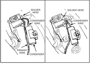
Fig. 26 - REPLACING CONDENSER WIRE
