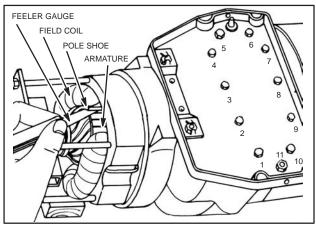
Fig. 168 – ALIGNING MODEL "WMG" GENERATOR
