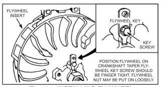
Fig. 69 - INSTALLING FLYWHEEL
