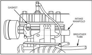
Fig. 231 – BREATHER TUBE AND INTAKE MANIFOLD, TYPICAL
