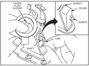
Fig. 165 - INSERTING CHOKE LINK
