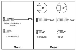
Fig. 286 - CHECKING NEEDLE VALVES
