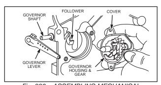
Fig. 336 – ASSEMBLING MECHANICAL GOVERNOR
