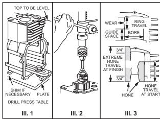
Fig. 819 – HONING CYLINDER (SEE PAGE 3 FOR ENLARGED DRAWING.)
