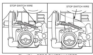
Fig. 171 - STOP SWITCH WIRES
