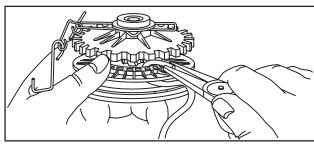
Fig. 622 - REMOVING ROPE FROM PULLEY
