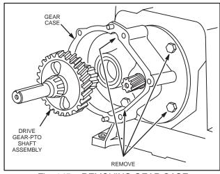
Fig. 145 - REMOVING GEAR CASE
