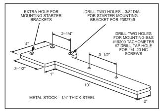
Fig. 645 - STARTER MOUNTING TEST BRACKET
