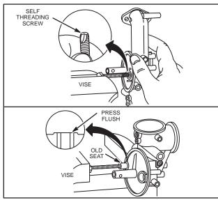
Fig. 263 - REPLACING FLOAT VALVE SEAT
