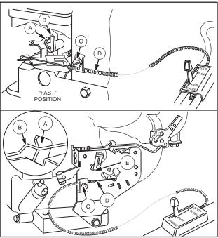
Fig. 355 – CHOKE-A-MATIC® CONTROL, TYPICAL
