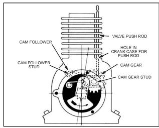
Fig. 534 - VALVE TIMING
