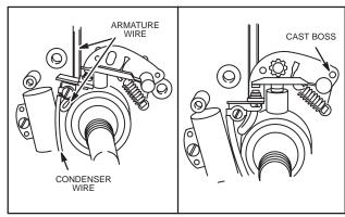
Fig. 32 - BREAKER POINTS WIRE ROUTING
