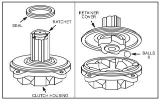
Fig. 610 – SEALED CLUTCH ASSEMBLY (CURRENT STYLE)
