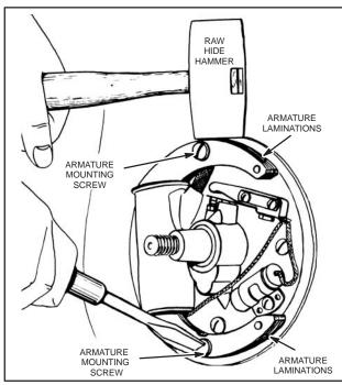
Fig. 24 - ADJUSTING ARMATURE AIR GAP
