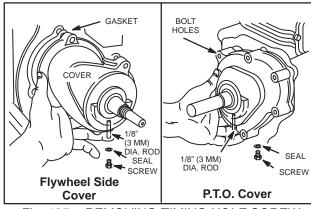
Fig. 185 - REMOVING TIMING HOLE SCREW
