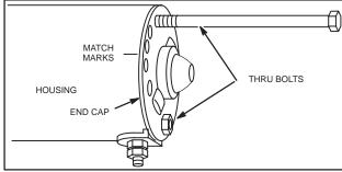
Fig. 670 - REMOVING THRU BOLTS
