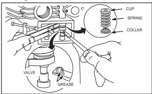
Fig. 510 - REMOVING SPRING
