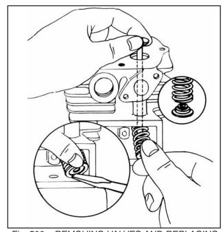
Fig. 500 – REMOVING VALVES AND REPLACING VALVES
