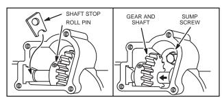
Fig. 154 – REMOVE AND INSTALL SUMP SCREW
