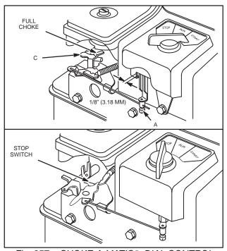
Fig. 357 – CHOKE-A-MATIC® DIAL CONTROL ADJUSTMENTS
