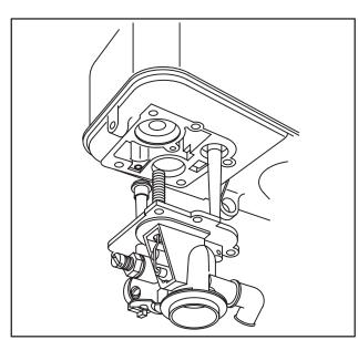
Fig. 243 - ASSEMBLING TANK TO **CARBURETOR**
