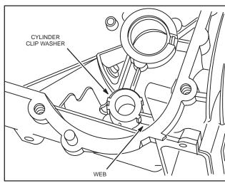
Fig. 167 - CYLINDER CLIP WASHER
