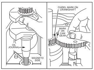
Fig. 888 - ALIGNING TIMING MARKS
