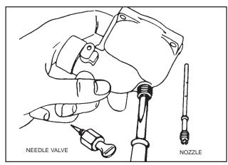
Fig. 272 - REMOVING NOZZLE
