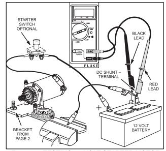
Fig. 667 - TESTING 12 VOLT STARTER MOTOR WITH DIGITAL MULTIMETER
