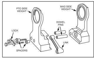
Fig. 190 – DISASSEMBLING COUNTERWEIGHT
