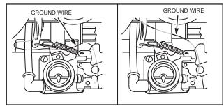
Fig. 214 - STOP SWITCH WIRES
