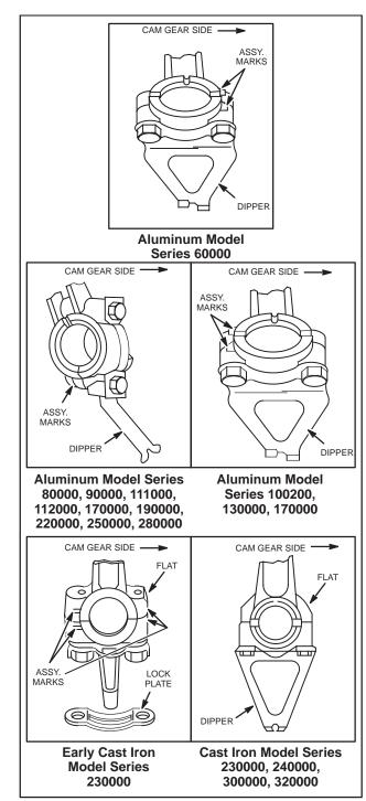
Fig. 576 – CONNECTING ROD INSTALLATION, HORIZONTAL CRANKSHAFT ENGINES
