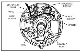
Fig. 53 - REMOVING BREAKER POINTS
