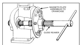
Fig. 910 – REAMING MAGNETO BEARING (LINE REAMING)
