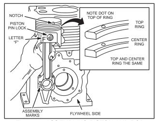
Fig. 547 - ASSEMBLING PISTON AND ROD
