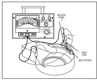
Fig. 784 – TESTING RECTIFIER
