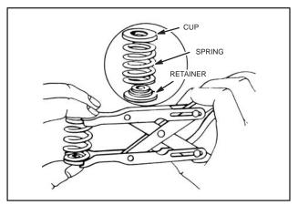
Fig. 506 - REMOVING VALVES
