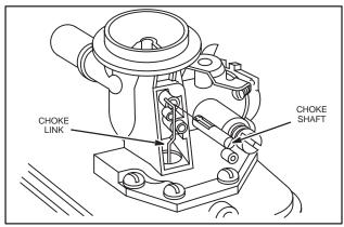
Fig. 144 – REMOVING AUTOMATIC CHOKE, TYPICAL
