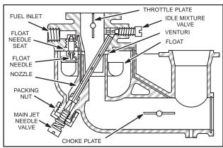
Fig. 269 – TYPICAL TWO PIECE FLO-JET CARBURETOR
