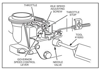
Fig. 174 - ADJUSTING CARBURETOR
