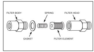
Fig. 301 - ELEMENT ASSEMBLY
