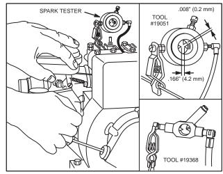
Fig. 5 - CHECKING IGNITION
