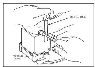
Fig. 579 - EXTENDED OIL FILL TUBE AND **DIPSTICK**
