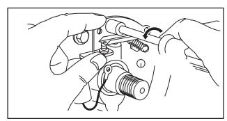
Fig. 85 - REMOVING STYLE II BREAKER POINTS
