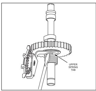
Fig. 160 - REMOVE CLUTCH SPRING
