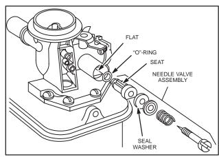
Fig. 247 – NEEDLE VALVE ASSEMBLY, PRESSED-IN TYPE
