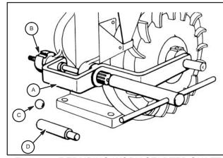
Fig. 587 - REPAIRING WORN STARTER SHAFT HOLE
