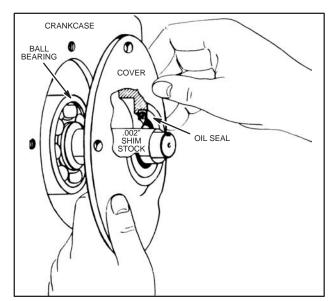
Fig. 891 - PROTECTING OIL SEAL
