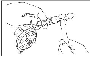
Fig. 611 - DISASSEMBLING SEALED CLUTCH
