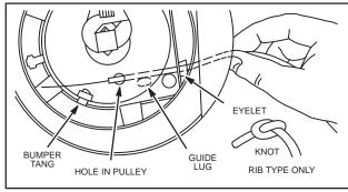
Fig. 606 - INSERTING ROPE, OLD STYLE
