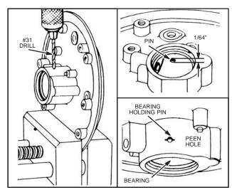
Fig. 905 - PINING BEARING
