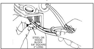
Fig. 505 - REMOVING VALVES
