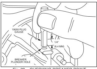
Fig. 92 – CHECKING BREAKER POINT PLUNGER HOLE
