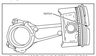
Fig. 546 – ASSEMBLING PISTON AND ROD
