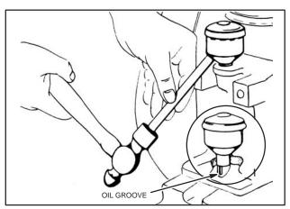
Fig. 173 - REMOVING BREATHER
