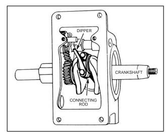
Fig. 557 - GENERAL VIEW OF ROD ASSEMBLY
