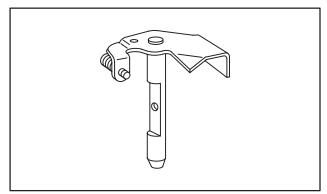
Fig. 237 – THROTTLE SHAFT AND LEVER, TYPICAL
