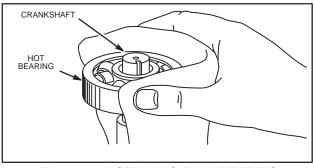
Fig. 918 - INSTALLING BALL BEARING
