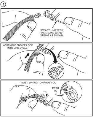
Fig. 333 - ASSEMBLE SPRING TO LINK EYELET
