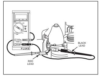
Fig. 741 – TESTING RECTIFIER
