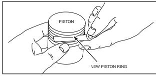
Fig. 542 - CHECKING RING GROOVES
