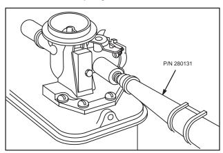
Fig. 248 - ASSEMBLING PRESSED-IN VALVE
