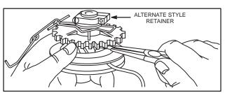
Fig. 623 - (ALTERNATE STYLE) REMOVING ROPE FROM PULLEY
