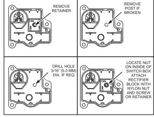
Fig. 707 – REPLACING RECTIFIER
