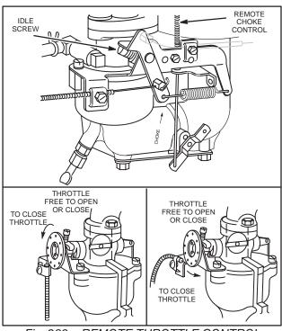
Fig. 283 - REMOTE THROTTLE CONTROL
