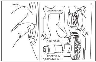
Fig. 869 - REMOVE CRANKSHAFT
