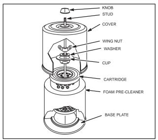
Fig. 116 – DUAL ELEMENT, HORIZONTAL AND VERTICAL CRANKSHAFT
