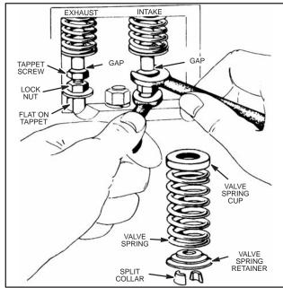
Fig. 496 - ADJUSTING VALVE CLEARANCE
