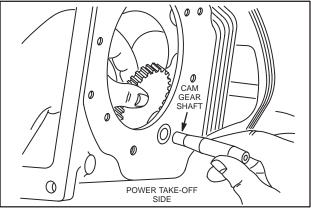
Fig. 885 - INSTALLING CAMSHAFT
