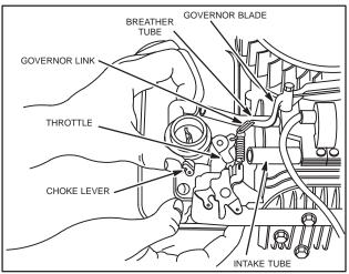
Fig. 170 – INSTALL CARBURETOR AND TANK ASSEMBLY
