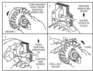
Fig. 104 - ADJUSTING IGNITION ARMATURE AIR GAP
