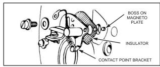
Fig. 31 - REPLACING BREAKER POINTS
