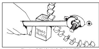
Fig. 8 - REMOVING FLYWHEEL
