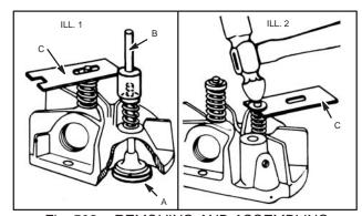
Fig. 508 – REMOVING AND ASSEMBLING VALVES MODEL FH
