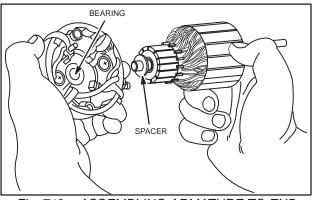
Fig. 712 – ASSEMBLING ARMATURE TO END CAP
