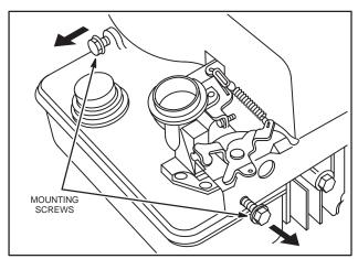
Fig. 220 - REMOVING MOUNTING SCREWS
