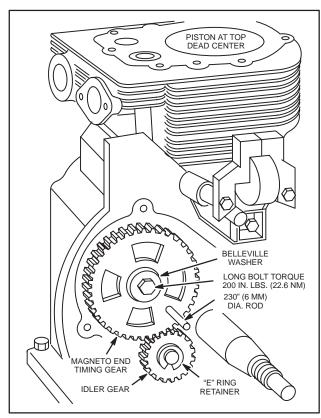
Fig. 183 – INSTALLING AND TIMING MAGNETO DRIVE GEAR
