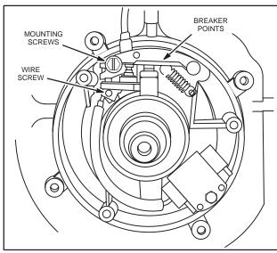
Fig. 91 – REMOVING STYLE III BREAKER POINTS
