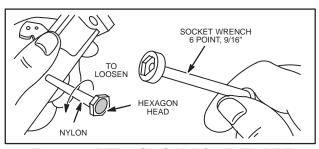
133 - REPLACING NYLON FUEL PIPE
