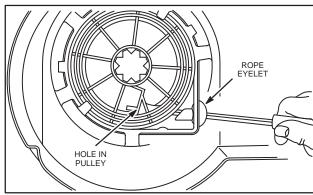
Fig. 607 – INSERTING ROPE
