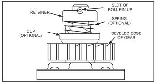
Fig. 694 – ASSEMBLING STARTER MOTOR DRIVE
