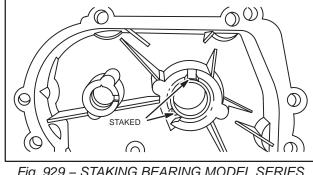
Fig. 929 – STAKING BEARING MODEL SERIES 6BH, 8BH, 60000, 80000, 90000, 100200, 100900, 110000, 120000, 130000, SUMP
