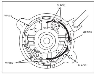
Fig. 710 - END CAP WIRING 120 VOLT AC
