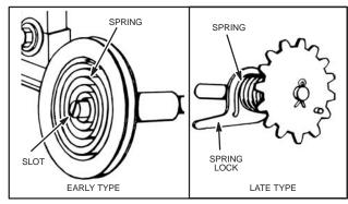
Fig. 581 – ADJUSTING SPRING TENSION
