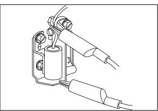
Fig. 73 – CONNECTING DIGITAL MULTIMETER #19357
