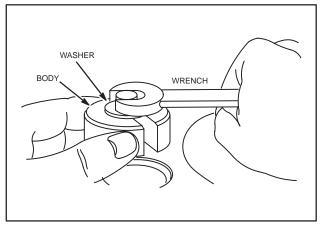
Fig. 524 - REMOVING VALVE SEAT
