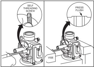
Fig. 287 - REPLACING FLOAT VALVE SEAT
