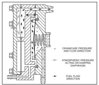
Fig. 311 – FUEL FLOW WITH CRANKCASE PRESSURE, TYPICAL
