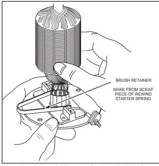
Fig. 673 – ASSEMBLING ARMATURE TO END CAP
