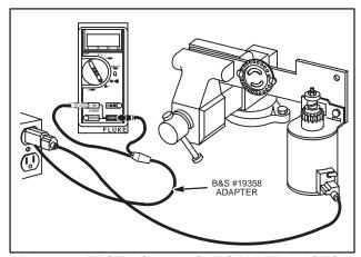
Fig. 682 - TESTING 120 VOLT STARTER MOTOR DIGITAL MULTIMETER
