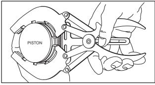
Fig. 541 - REMOVING RINGS
