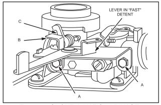
Fig. 254 - CHOKE-A-MATIC® LINKAGE - MODEL SERIES 100900, 130900, 131900
