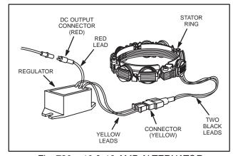
Fig. 780 - 10 & 16 AMP ALTERNATOR **ASSEMBLY**
