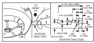
Fig. 638 - REMOVING SPRING HOUSING
