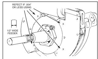
Fig. 50 - CHECKING FOR WEAR
