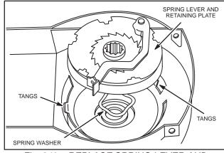
Fig. 640 – REPLACE SPRING LEVER AND RETAINING PLATE
