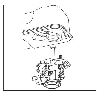
Fig. 164 – ASSEMBLING TANK TO **CARBURETOR**
