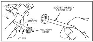
Fig. 186 – INSTALLING NYLON FUEL PICK-UP TUBE
