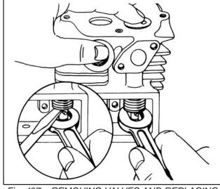
Fig. 497 – REMOVING VALVES AND REPLACING VALVES
