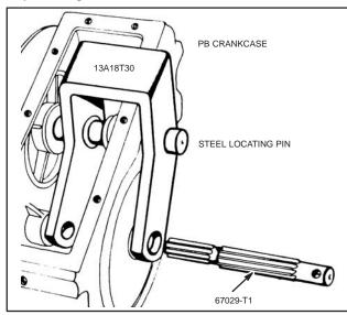
Fig. 916 – REAMING MODELS D, P, PB CAM BEARING
