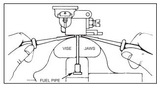
134 - REMOVING BRASS FUEL PIPE
