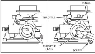
Fig. 238 - INSTALLING THROTTLE, TYPICAL
