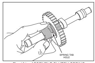
Fig. 161 - ASSEMBLE CLUTCH SPRING
