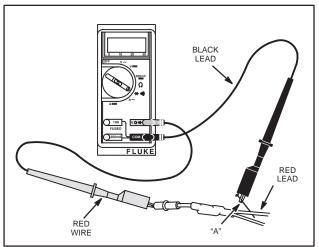
Fig. 769 – DIODE TESTING – CHARGING CIRCUIT
