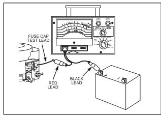
Fig. 747 - TESTING ALTERNATOR OUTPUT
