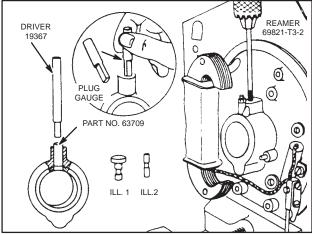
Fig. 19 – INSTALLING BREAKER POINT BUSHING
