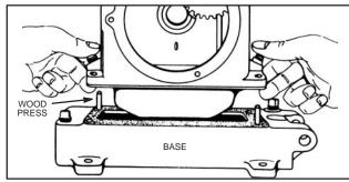
Fig. 565 - MOUNTING CRANKCASE MODEL FH
