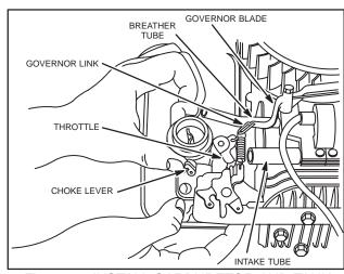
Fig. 249 - INSTALL CARBURETOR AND TANK **ASSEMBLY**
