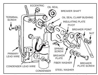
Fig. 40 - REMOVING BREAKER POINTS
