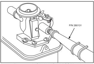
Fig. 169 – INSTALLING PRESSED-IN NEEDLE VALVE
