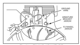
Fig. 74 - TIMING ARMATURE
