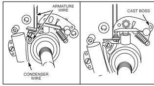
Fig. 88 - ADJUSTING STYLE I BREAKER POINTS
