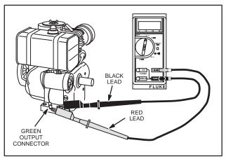
Fig. 768 – TESTING ALTERNATOR OUTPUT
