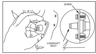
Fig. 872 - REMOVING CAM GEAR BEARING
