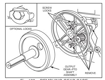
Fig. 138 - REMOVING GEAR CASE
