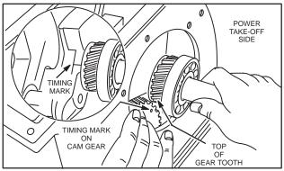
Fig. 887 - TIMING CRANKSHAFT
