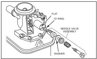
Fig. 227 – NEEDLE VALVE ASSEMBLY, PRESSED-IN-TYPE
