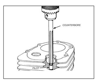
Fig. 529 - COUNTERBORING FOR VALVE GUIDE
