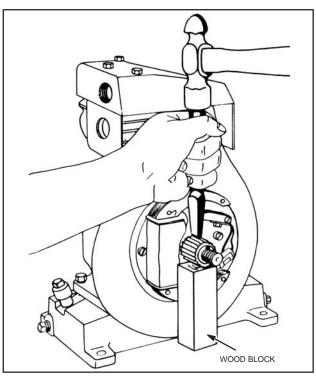
Fig. 116 - REMOVING FLYWHEEL HUB
