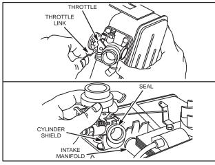
Fig. 223 – REMOVING CARBURETOR MODEL SERIES 100900, 130900, 131900, VERTICAL CRANKSHAFT
