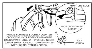
Fig. 72 - TIMING ARMATURE
