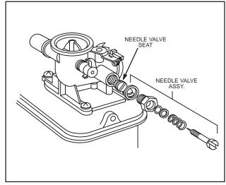
Fig. 211 – NEEDLE VALVE ASSEMBLY, ZINC BODY
