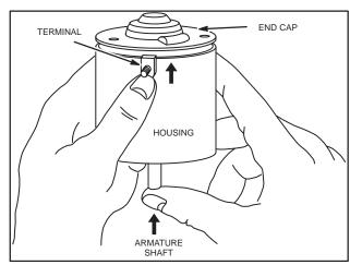
Fig. 671 – REMOVING ARMATURE
