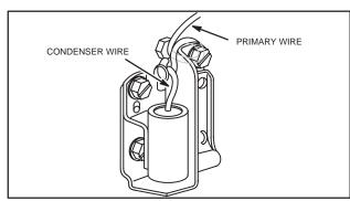
Fig. 67 – INSTALLING PRIMARY WIRE AND CONDENSER
