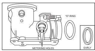
Fig. 226 – METERING HOLES AND "O"-RING, TYPICAL
