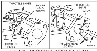
Fig. 149 – REMOVING THROTTLE PLATE, TYPICAL
