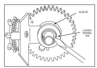
Fig. 159 - REMOVE CLUTCH SLEEVE
