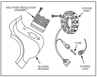
Fig. 734 - ALTERNATOR ASSEMBLY
