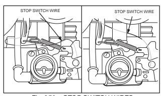
Fig. 250 – STOP SWITCH WIRES
