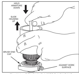
Fig. 700 - REMOVING MOTOR HOUSING
