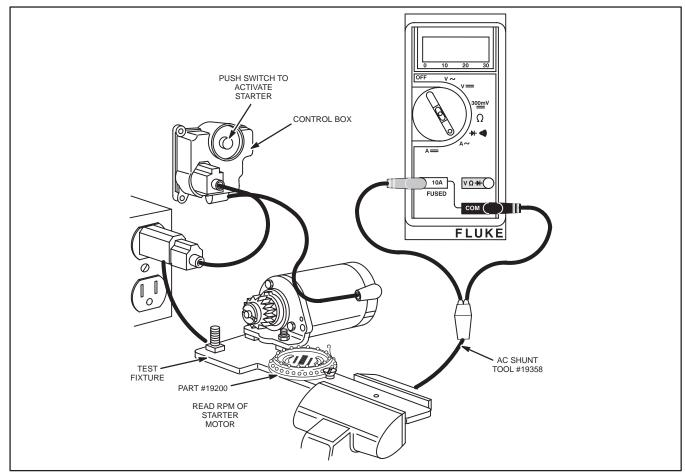
Fig. 697 - TESTING 120 VOLT AC STARTER - DIGITAL MULTIMETER
