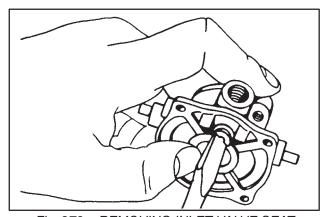
Fig. 273 - REMOVING INLET VALVE SEAT
