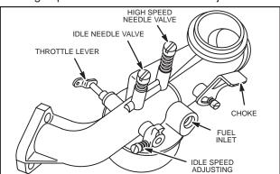
Fig. 256 – SMALL ONE-PIECE FLO-JET CARBURETOR
