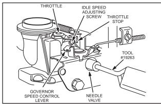
Fig. 255 - ADJUSTING CARBURETOR
