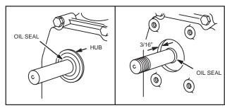
Fig. 821 - REPLACING OIL SEAL
