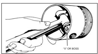
Fig. 544 - ASSEMBLING CONNECTING ROD
