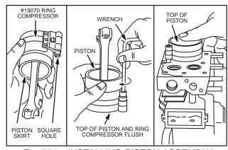
Fig. 554 - INSTALLING PISTON ASSEMBLY
