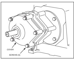
Fig. 144 – DRAINING GEAR REDUCTION AND REMOVING COVER
