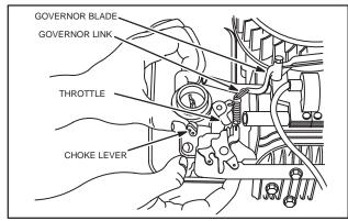
Fig. 213 – INSTALL CARBURETOR AND TANK ASSEMBLY
