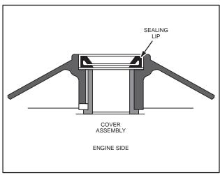
Fig. 147 - INSTALLING SEAL
