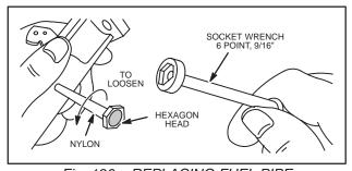
Fig. 196 - REPLACING FUEL PIPE
