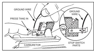
Fig. 190 - REMOVING GROUND WIRE
