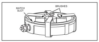
Fig. 686 - INSERTING BRUSHES
