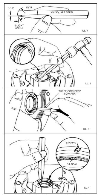
Fig. 914 - REMOVING & REPLACING OIL SEAL
