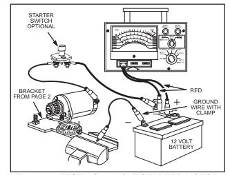
Fig. 681 – TESTING 12 VOLT STARTER MOTOR VOA METER
