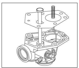
Fig. 163 - LOCATING DIAPHRAGM ON **CARBURETOR**
