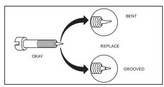
Fig. 181 - MIXTURE NEEDLE
