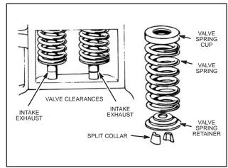
Fig. 494 - CHECKING AND ADJUSTING VALVES
