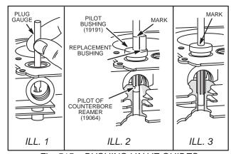
Fig. 515 - BUSHING VALVE GUIDES
