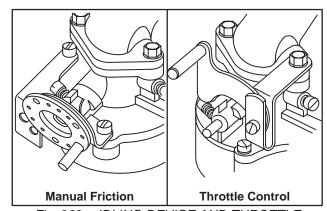
Fig. 282 – IDLING DEVICE AND THROTTLE CONTROL
