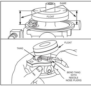
Fig. 265 - CHECKING FLOAT LEVEL
