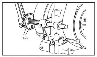
Fig. 580 - ADJUSTING SPRING TENSION
