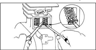
Fig. 504 - REMOVING VALVES
