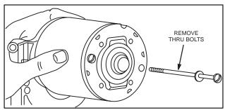
Fig. 655 - REMOVING THRU BOLTS
