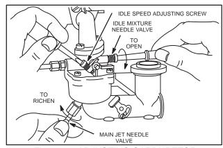
Fig. 281 - ADJUSTING CARBURETOR
