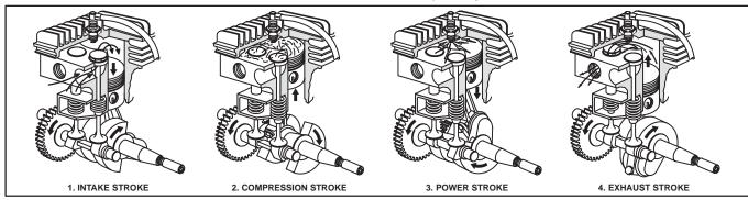
Fig. 1 – THE 4-STROKE CYCLE
