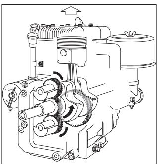
Fig. 186 – ALUMINUM ENGINES, ROTATING COUNTERBALANCE SYSTEM
