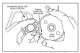
Fig. 889 - BALL BEARING ENGINES
