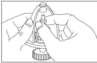
Fig. 666 - ASSEMBLING STARTER MOTOR DRIVE
