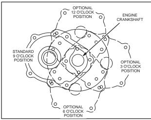
Fig. 148 – POSITIONING GEAR CASE ASSEMBLY
