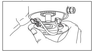
Fig. 687 – INSTALLING END CAP
