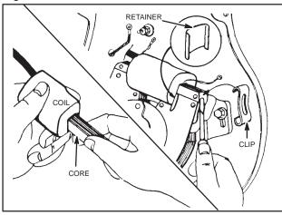
Fig. 42 – REMOVING COIL
