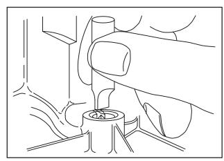
Fig. 932 - CHECKING CAM GEAR BEARING
