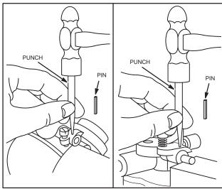
Fig. 275 – REMOVE THROTTLE SHAFT AND BUSHINGS
