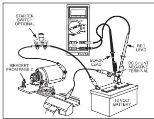
Fig. 680 – TESTING 12 VOLT STARTER MOTOR
