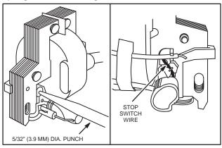
Fig. 102 - REMOVING STOP SWITCH WIRE
