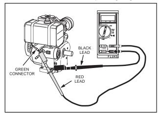
Fig. 775 - TESTING ALTERNATOR OUTPUT
