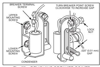
Fig. 57 - REMOVING BREAKER POINTS
