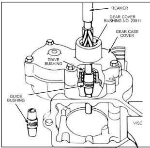
Fig. 117 - INSERTING GUIDE BUSHING
