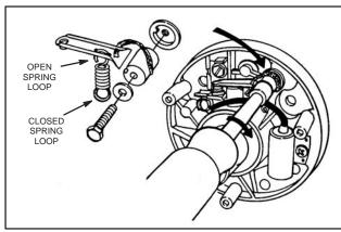
Fig. 55 - INSTALLING BREAKER POINTS
