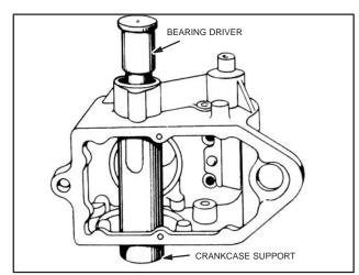
Fig. 908 - REMOVING DRIVE BEARING
