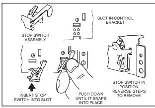
Fig. 106 – TYPICAL STOP SWITCH INSTALLATION
