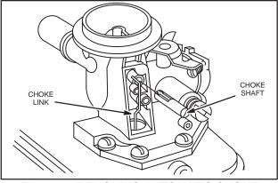
Fig. 225 – REMOVING AUTOMATIC CHOKE, TYPICAL
