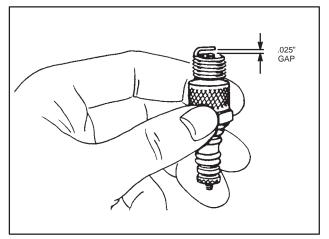
Fig. 2 - CHECKING SPARK GAP
