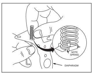
Fig. 241 – ASSEMBLING SPRING TO DIAPHRAGM
