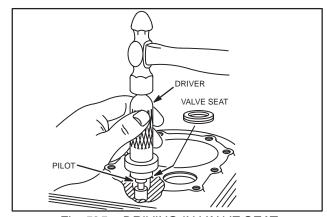
Fig. 525 - DRIVING IN VALVE SEAT
