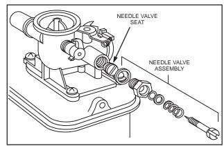
Fig. 167 – NEEDLE VALVE ASSEMBLY, SCREW-IN TYPE
