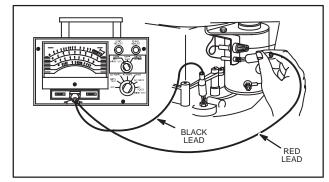
Fig. 785 - TESTING AC OUTPUT
