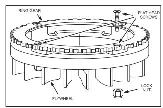
Fig. 690 - REPLACING RING GEAR
