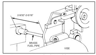
Fig. 135 - REPLACING BRASS FUEL PIPE
