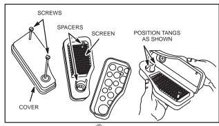
Fig. 120 – OIL-FOAM<sup>®</sup> AIR CLEANER, VERTICAL CRANKSHAFT
