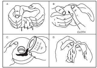
Fig. 122 - CLEANING OIL-FOAM® AIR CLEANER
