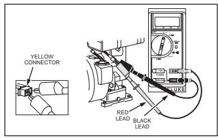
Fig. 771 – TESTING ALTERNATOR OUTPUT
