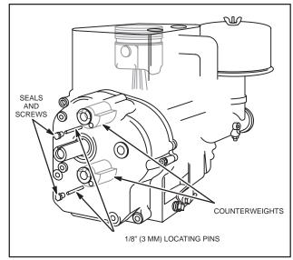
Fig. 187 – TIMING COUNTERBALANCE GEARS
