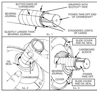
Fig. 912 - PROTECTING OIL SEAL
