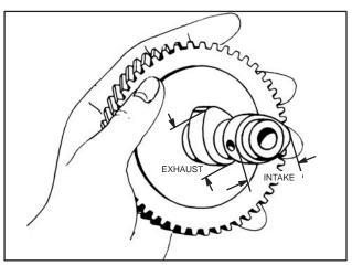
Fig. 876 - CAM GEAR CHECK POINTS
