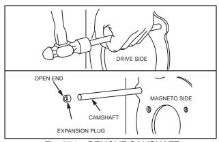
Fig. 874 - REMOVE CAMSHAFT
