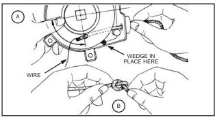
Fig. 594 – INSTALL ROPE IN PULLEY AND TIE **KNOT**
