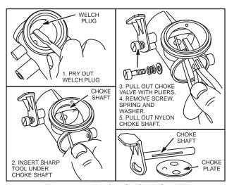
Fig. 261 – NYLON CHOKE SHAFT
