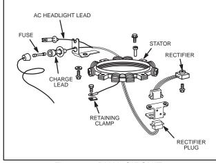
Fig. 729 – DUAL CIRCUIT – FUSED (EARLY STYLE)
