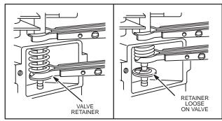
Fig. 512 - REMOVING RETAINER AND SPRING
