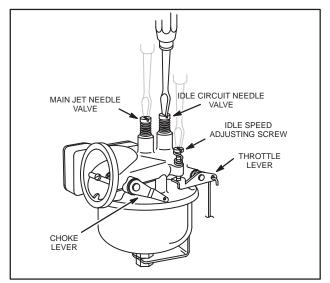
Fig. 293 - CARBURETOR ADJUSTMENT
