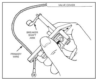
Fig. 41 – REMOVING BREAKER BOX
