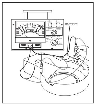
Fig. 749 - TESTING RECTIFIER
