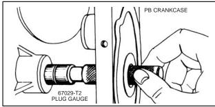
Fig. 915 – GAUGING MODELS D, P, PB CAM BEARING
