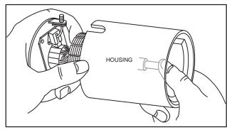
Fig. 674 - INSERTING ARMATURE
