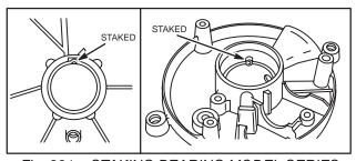
Fig. 931 – STAKING BEARING MODEL SERIES 140000, 190000, 220000, 250000 CYLINDER OR CRANKCASE COVER
