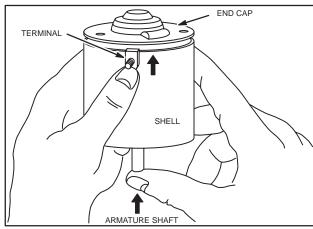
Fig. 656 - REMOVING ARMATURE
