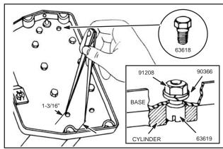
Fig. 169 – ALIGNING MODEL "WMG" GENERATOR
