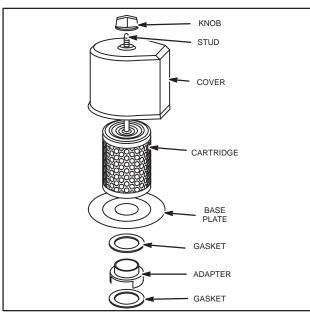
Fig. 115 – CARTRIDGE TYPE, HORIZONTAL AND VERTICAL CRANKSHAFT
