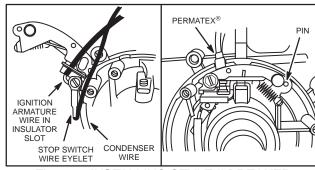
Fig. 97 – INSTALLING STYLE II BREAKER POINTS
