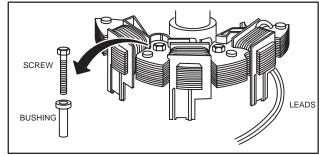
Fig. 744 - ASSEMBLING STATOR
