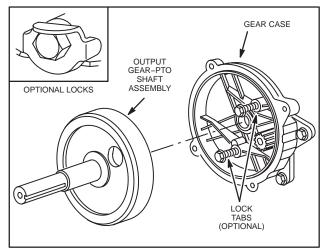
Fig. 131 – REMOVING DRIVE GEAR AND GEAR CASE
