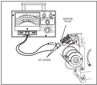
Fig. 778 - TESTING ALTERNATOR OUTPUT
