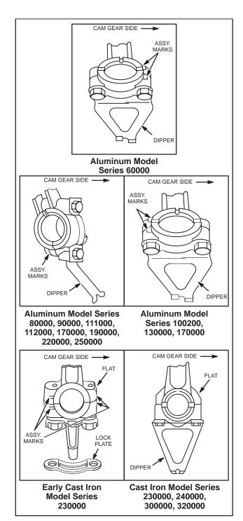
Fig. 181 – CONNECTING ROD INSTALLATION, HORIZONTAL CRANKSHAFT ENGINES
