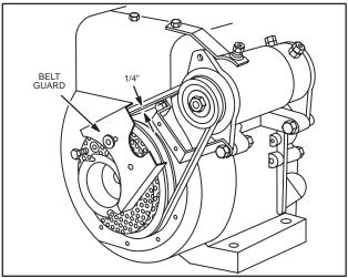
Fig. 717 – 12 VOLT STARTER – GENERATOR (HIGH POSITION)
