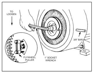
Fig. 7 - REMOVING FLYWHEEL
