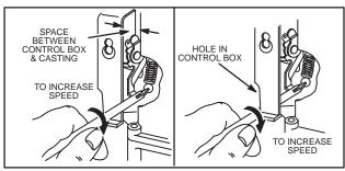
Fig. 347 - ADJUSTING TOP-NO-LOAD RPM
