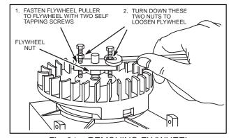
Fig. 81 – REMOVING FLYWHEEL
