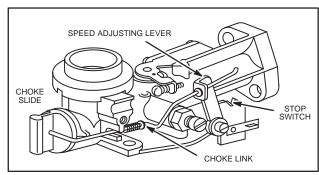
Fig. 200 - CHOKE-A-MATIC® LINKAGE
