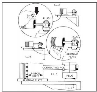
Fig. 548 - ALIGNING ROD AND PISTON
