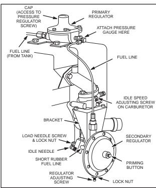
Fig. 300 – ADJUSTING CARBURETOR, LP FUEL SYSTEM
