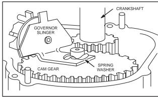
Fig. 578 - OIL SLINGER AND BRACKET VERTICAL CRANKSHAFT ENGINES
