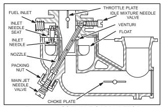
Fig. 280 - ASSEMBLE CARBURETOR
