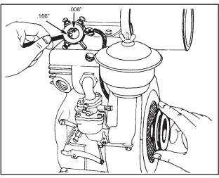
Fig. 4 - CHECKING SPARK
