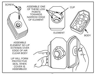
Fig. 119 – OIL-FOAM<sup>®</sup> AIR CLEANER, HORIZONTAL AND VERTICAL CRANKSHAFT
