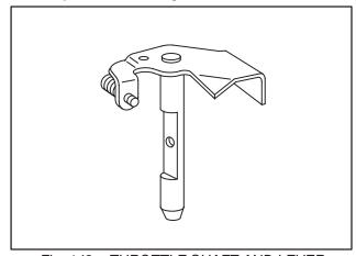
Fig. 148 - THROTTLE SHAFT AND LEVER
