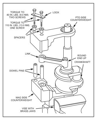
Fig. 191 – ASSEMBLING COUNTERWEIGHT TO CRANKSHAFT
