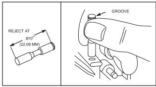
Fig. 99 – CHECKING BREAKER POINT PLUNGER HOLE
