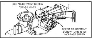
Fig. 207 - SETTING NEEDLE VALVE
