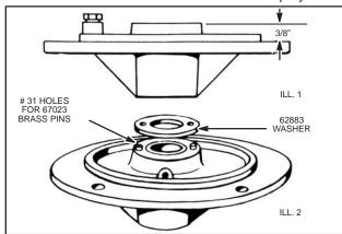
Fig. 113 - REPAIRING WORN THRUST FACE
