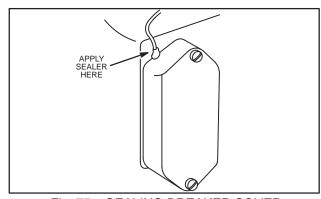
Fig. 75 - SEALING BREAKER COVER
