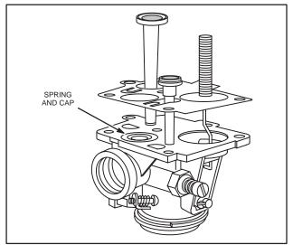
Fig. 242 - LOCATING DIAPHRAGM ON **CARBURETOR**
