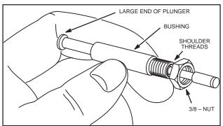
Fig. 65 - INSERTING PLUNGER INTO BUSHING
