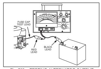
Fig. 762 - TESTING ALTERNATOR OUTPUT
