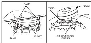
Fig. 289 - CHECKING FLOAT LEVEL
