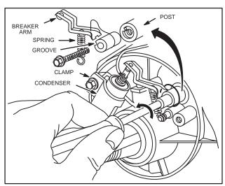
Fig. 89 - REMOVING STYLE II BREAKER POINTS
