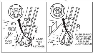
Fig. 514 - INSTALLING VALVES
