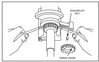
Fig. 189 - REMOVING CRANKSHAFT GEAR
