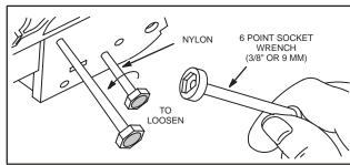
Fig. 230 – REMOVING NYLON FUEL PICK-UP TUBES
