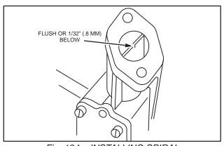
Fig. 184 – INSTALLING SPIRAL
