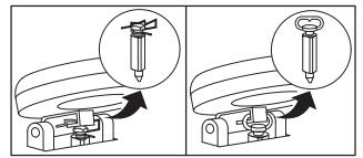
Fig. 264 - INLET NEEDLE VALVE VARIATIONS
