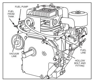
Fig. 310 - VACUUM FROM HOLLOW BOLT
