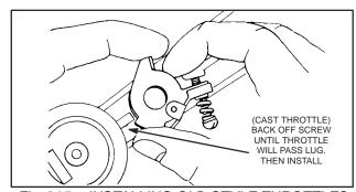
Fig. 205 - INSTALLING OLD STYLE THROTTLES
