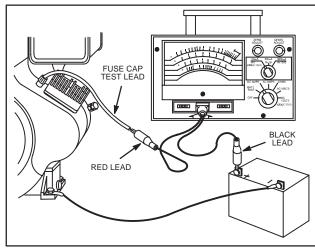
Fig. 779 - TESTING REGULATOR - RECTIFIER
