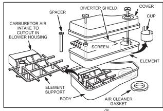
Fig. 121 – DUCTED OIL-FOAM<sup>®</sup> AIR CLEANER, VERTICAL CRANKSHAFT
