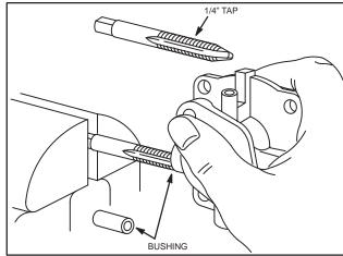
Fig. 276 – REPLACING THROTTLE SHAFT BUSHINGS
