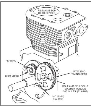
Fig. 184 – INSTALLING AND TIMING PTO DRIVE GEAR
