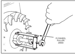
Fig. 11 - REMOVING FLYWHEEL
