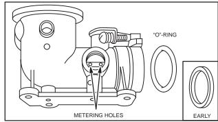
Fig. 146 – METERING HOLES AND "O"-RING, TYPICAL
