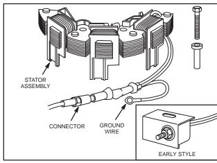
Fig. 738 - ALTERNATOR ASSEMBLY
