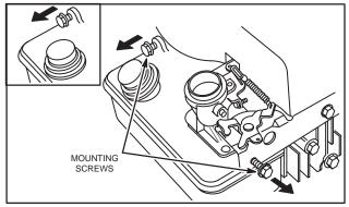
Fig. 188 - REMOVING MOUNTING BOLTS
