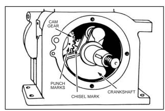
Fig. 532 - VALVE TIMING
