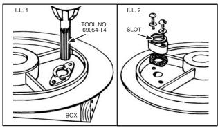
Fig. 171 - REPLACING OIL RETURN VALVE
