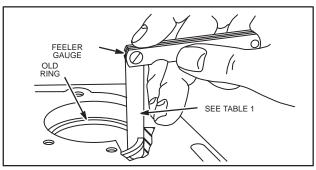
Fig. 543 - CHECKING RING GAP
