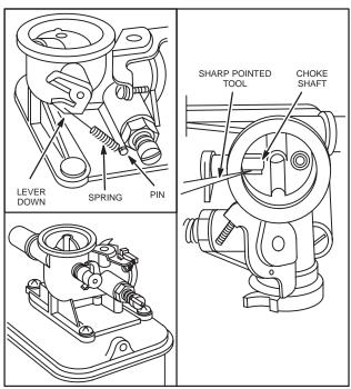
Fig. 152 – CHOKE SHAFT AND VALVE – CHOKE-A-MATIC®
