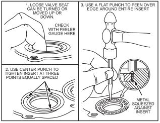
Fig. 526 - PEENING VALVE SEAT
