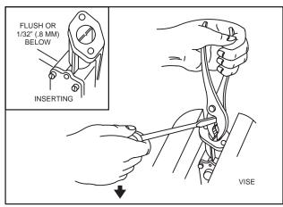
Fig. 194 - REMOVING AND INSERTING SPIRAL
