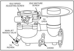
Fig. 268 – LARGE FLO-JET, HORIZONTAL CRANKSHAFT
