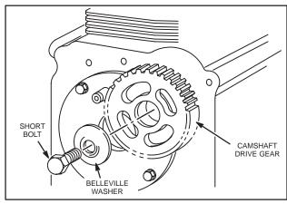
Fig. 870 - REMOVE SHORT BOLT
