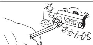
Fig. 9 - REMOVING FLYWHEEL
