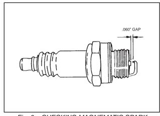
Fig. 6 - CHECKING MAGNEMATIC SPARK
