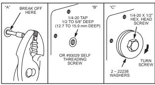
Fig. 60 - REMOVING BUSHING AND PLUNGER
