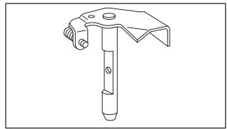
Fig. 177 – THROTTLE SHAFT AND LEVER, TYPICAL
