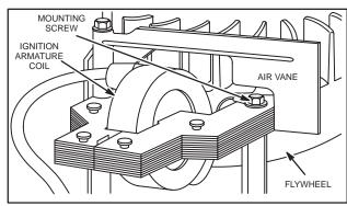
Fig. 100 – INSTALLING IGNITION ARMATURE AND AIR VANE, (TYPICAL)
