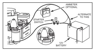
Fig. 739 - TYPICAL WIRING INSTALLATION
