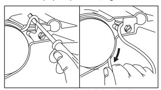
Fig. 634 - ADDING TENSION TO ROPE
