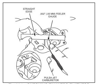
Fig. 234 - CHECKING TANK TOP FLATNESS
