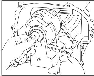
Fig. 192 – INSTALLING CRANKSHAFT AND COUNTERWEIGHT ASSEMBLY
