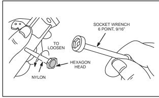
Fig. 156 – INSTALLING FUEL PICK-UP TUBE, TYPICAL
