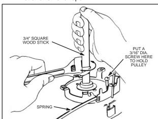
Fig. 588 - REMOVING ROPE
