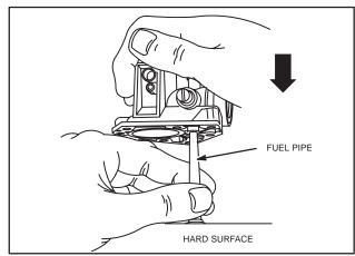
Fig. 157 – INSTALLING FUEL PIPE, MINLON ™ CARBURETOR
