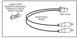
Fig. 773 - TEST EQUIPMENT
