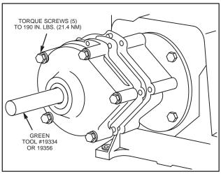
Fig. 149 – INSTALLING GEAR CASE COVER ASSEMBLY
