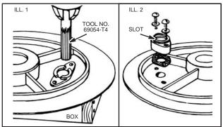
Fig. 170 - REPLACING OIL RETURN VALVE
