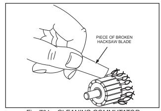
Fig. 701 - CLEANING COMMUTATOR
