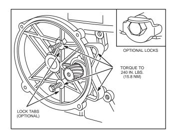
Fig. 141 - INSTALLING GEAR CASE
