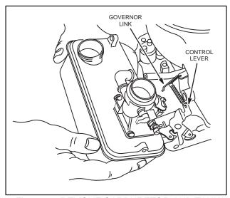
Fig. 189 – REMOVE CARBURETOR AND TANK ASSEMBLY
