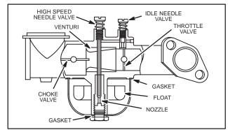
Fig. 257 – SMALL ONE-PIECE FLO-JET CARBURETOR
