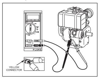
Fig. 781 - TESTING ALTERNATOR OUTPUT
