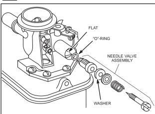
Fig. 147 – NEEDLE VALVE ASSEMBLY, PRESSED-IN-TYPE
