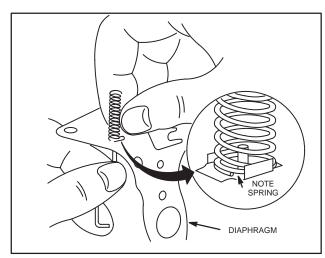
Fig. 160 – ASSEMBLE SPRING TO DIAPHRAGM
