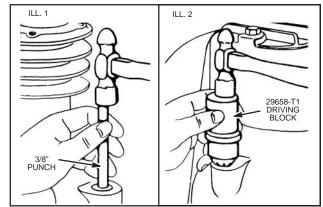
Fig. 176 - REPLACING BREATHER
