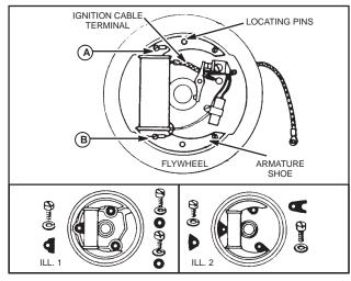
Fig. 27 - REPLACING ARMATURE
