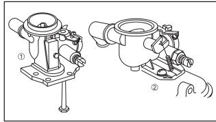
Fig. 141 – TYPES OF VACU-JET CARBURETORS
