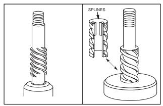
Fig. 679 – ASSEMBLING STARTER MOTOR DRIVE
