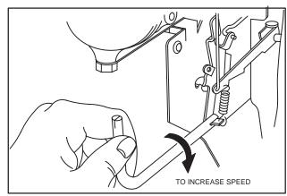
Fig. 352 - ADJUSTING TOP-NO-LOAD RPM
