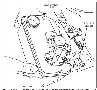
Fig. 221 – REMOVING CARBURETOR AND TANK ASSEMBLY
