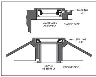
Fig. 139 - INSTALLING SEALS
