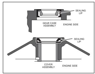
Fig. 132 - INSTALLING SEALS
