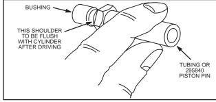
Fig. 66 - INSTALLING PLUNGER AND BUSHING
