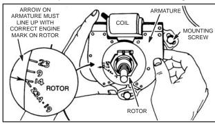
Fig. 49 – TIMING ROTOR
