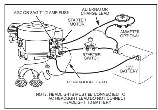
Fig. 761 – TYPICAL WIRING INSTALLATION
