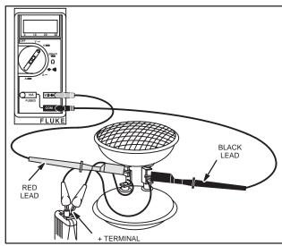
Fig. 650 – TESTING BATTERY WITH DIGITAL MULTIMETER
