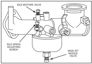
Fig. 258 – LARGE ONE-PIECE FLO-JET CARBURETOR
