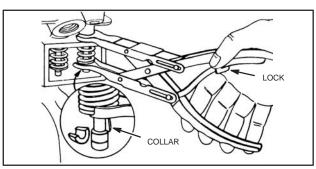
Fig. 503 - REMOVING VALVES
