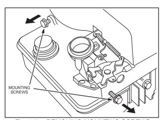
Fig. 142 - REMOVING MOUNTING SCREWS
