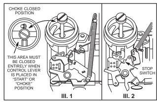
Fig. 356 - CHOKE AND STOP POSITION
