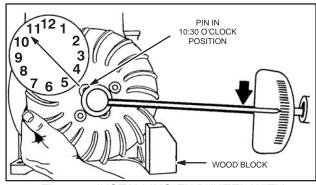
Fig. 51 – INSTALLING FLYWHEEL WITH STARTER PIN
