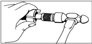
Fig. 522 - REMOVING CUTTER FROM SHANK
