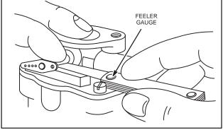
Fig. 271 - CHECKING THROTTLE WEAR
