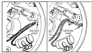
Fig. 17 - REPLACING CONDENSER
