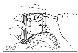
Fig. 36 - REPLACING ARMATURE
