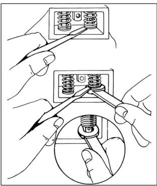
Fig. 501 – REMOVING VALVES AND REPLACING **VALVES**
