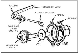
Fig. 323 – GOVERNOR HOUSING AND GEAR ASSEMBLY
