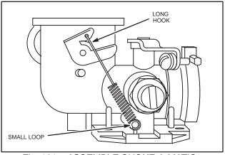
Fig. 161 - ASSEMBLE CHOKE-A-MATIC® **SPRING**
