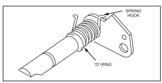
Fig. 164 - ASSEMBLE SPRING
