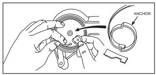
Fig. 628 - INSTALLING SPRING ANCHOR
