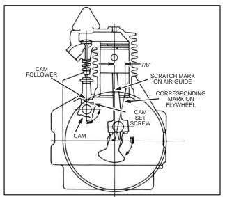
Fig. 533 - VALVE TIMING
