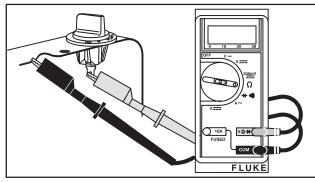
Fig. 107 - CHECKING ROTARY STOP SWITCH
