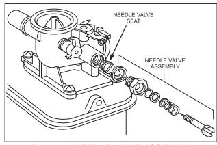
Fig. 246 – NEEDLE VALVE ASSEMBLY, SCREW-IN TYPE
