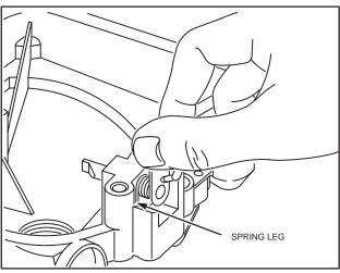
Fig. 166 - SPRING INSTALLATION
