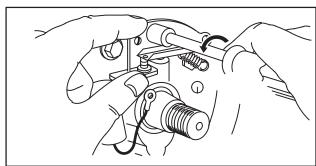
Fig. 30 – REMOVING BREAKER POINTS
