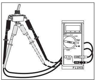
Fig. 109 – CHECKING MULTIPLE TERMINAL SWITCH
