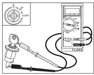
Fig. 110 - CHECKING METAL KEY SWITCH
