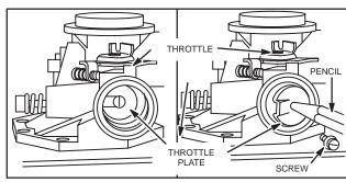
Fig. 229 - REMOVING THROTTLE, TYPICAL
