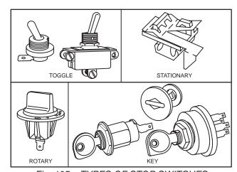
Fig. 105 - TYPES OF STOP SWITCHES
