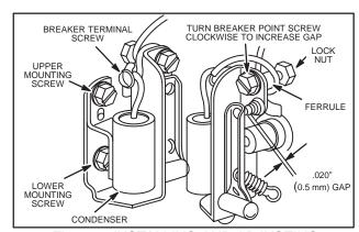
Fig. 68 – INSTALLING AND ADJUSTING BREAKER POINTS
