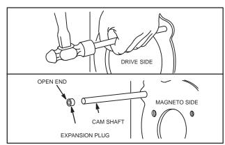
Fig. 868 - REMOVE CAMSHAFT
