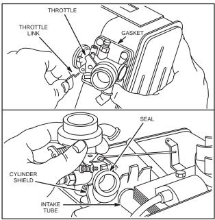
Fig. 251 – INSTALLING CARBURETOR MODEL SERIES 100900, 130900, 131900
