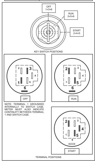
Fig. 111 - TESTING KEYSWITCH
