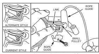
Fig. 630 - INSTALLING PULLEY ASSEMBLY
