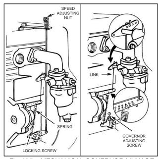
Fig. 325 – MECHANICAL GOVERNOR LINKAGE
