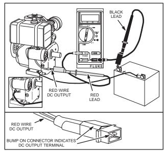
Fig. 766 - TESTING ALTERNATOR OUTPUT
