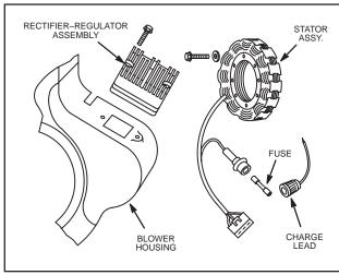
Fig. 777 - ALTERNATOR ASSEMBLY
