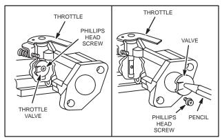
Fig. 193 - REMOVING STAMPED THROTTLE
