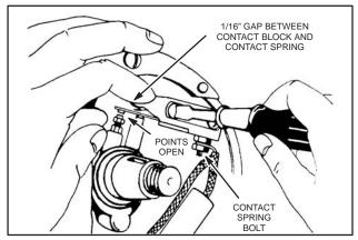
Fig. 15 - ADJUSTING POINT TENSION
