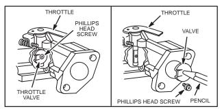
Fig. 206 – REMOVING AND INSTALLING NEW STYLE THROTTLES
