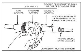
Fig. 875 – CRANKSHAFT CHECK POINTS
