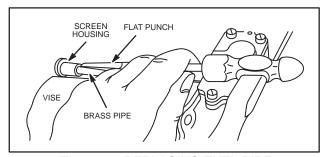
Fig. 197 - REPLACING FUEL PIPE
