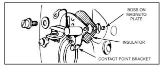
Fig. 86 - REPLACING BREAKER POINTS
