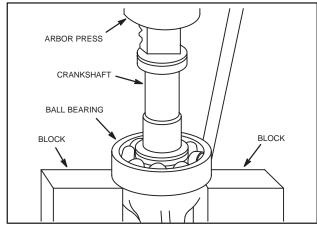
Fig. 917 - REMOVING BALL BEARINGS
