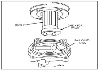
Fig. 609 - STARTER CLUTCH (OLD STYLE)
