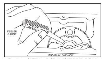
Fig. 893 - CHECKING CRANKSHAFT END PLAY
