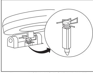
Fig. 288 – INSTALLING FLOAT AND INLET NEEDLE
