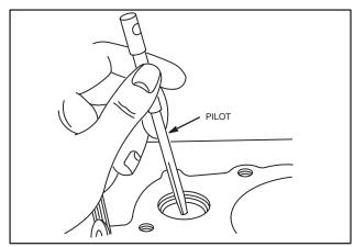
Fig. 519 - INSERTING PILOT
