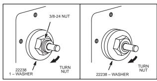
Fig. 64 - INSTALLING BUSHING AND PLUNGER
