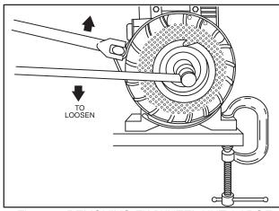
Fig. 80 – REMOVING FLYWHEEL NUT, LARGE FLYWHEELS
