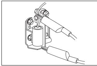
Fig. 70 – CONNECTING DIGITAL MULTIMETER #19357 OR VOA METER #19236
