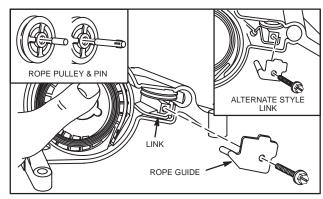
Fig. 620 - REMOVING ROPE GUIDE
