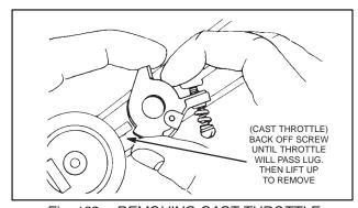
Fig. 192 - REMOVING CAST THROTTLE
