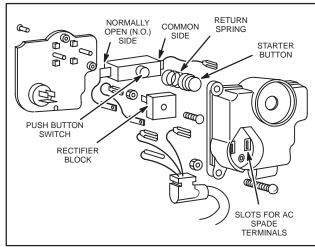
Fig. 703 – EXPLODED VIEW – CONTROL ASSEMBLY
