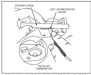
Fig. 155 - CHECKING TANK TOP FLATNESS
