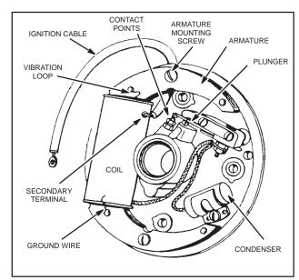
Fig. 18 – REPLACING ARMATURE
