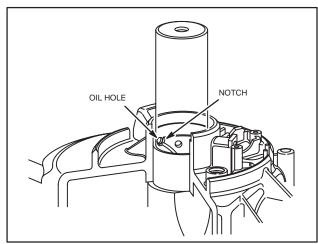
Fig. 924 – INSTALLING BUSHING MODEL SERIES 171700, 191700
