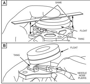
Fig. 279 A/B – CHECKING FLOAT LEVEL (LATER)
