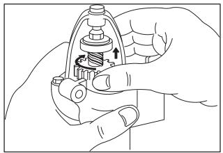
Fig. 665 – CHECKING STARTER MOTOR DRIVE
