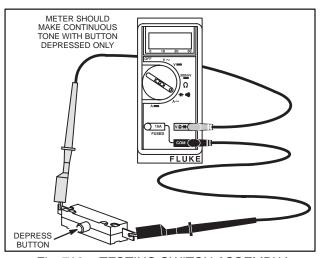
Fig. 708 - TESTING SWITCH ASSEMBLY
