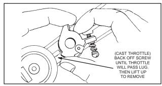
Fig. 130 - REMOVING OLD STYLE THROTTLES
