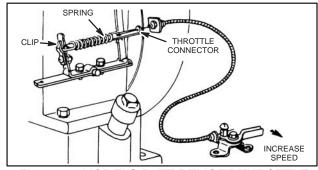
Fig. 365 – MODELS B, ZZ REMOTE THROTTLE CONTROL
