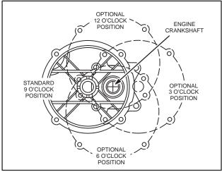
Fig. 133 – POSITIONING BEARING HOUSING ASSEMBLY
