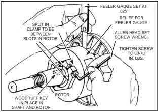
Fig. 44 - INSTALLING ROTOR (WITH CLAMP)
