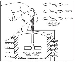
Fig. 818 - CHECKING CYLINDER BORE
