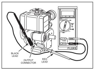
Fig. 759 - TESTING AC OUTPUT
