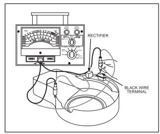
Fig. 755 - TESTING RECTIFIER
