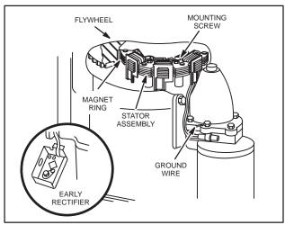
Fig. 743 - STATOR ASSEMBLY LOCATION
