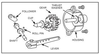
Fig. 335 - MECHANICAL GOVERNOR PARTS
