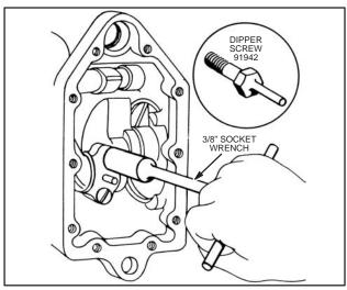
Fig. 575 - INSTALLING DIPPER SCREW
