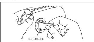
Fig. 919 - CHECKING BEARING
