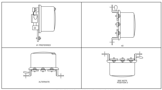
Fig. 720 – VOLTAGE REGULATOR MOUNTING POSITIONS
