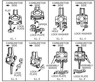
Fig. 545 - CONNECTING ROD INSTALLATION
