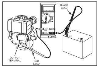
Fig. 757 - TESTING ALTERNATOR OUTPUT
