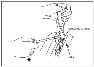
Fig. 176 - REMOVING SPIRAL
