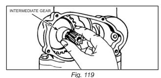
Put drive gear shaft through bearing in gear case
