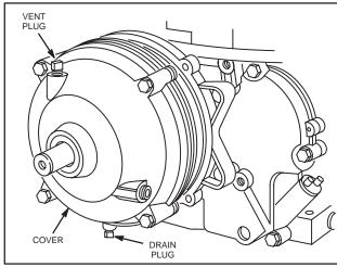
Fig. 137 – DRAINING GEAR REDUCTION AND REMOVING COVER
