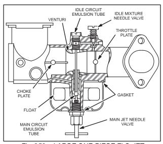
Fig. 259 – LARGE ONE-PIECE FLO-JET CARBURETOR
