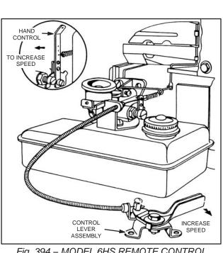
Fig. 394 - MODEL 6HS REMOTE CONTROL
