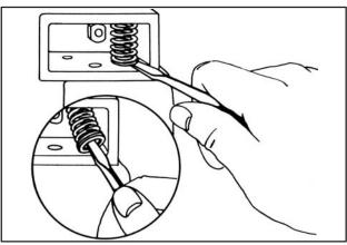
Fig. 499 – REMOVING VALVES AND REPLACING VALVES
