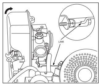
Fig. 222 - REMOVING FUEL TANK ASSEMBLY
