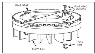
Fig. 677 - REPLACING RING GEAR
