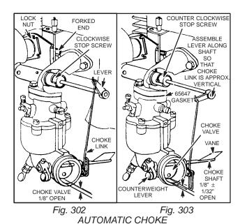
Rotate thermostat shaft counterclockwise until stop screw strikes the opposite side of tube, Fig. 303. Then open choke valve manually until it stops against the top of the choke link opening. The choke valve should now be open approximately 1/8" as before.
