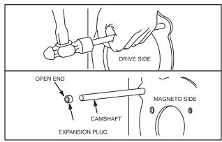
Fig. 880 - INSTALLING CAMSHAFT
