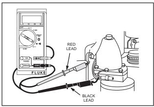
Fig. 742 - TESTING RECTIFIER
