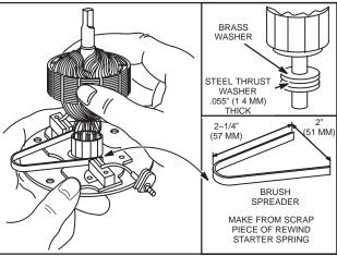
Fig. 658 – ASSEMBLING ARMATURE TO END CAP
