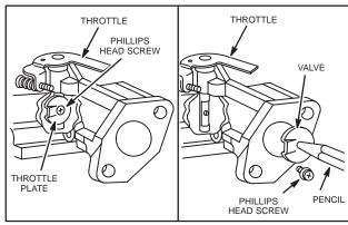
Fig. 183 - INSTALLING THROTTLE PLATE
