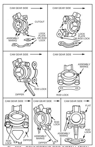
Fig. 556 – CONNECTING ROD INSTALLATION
