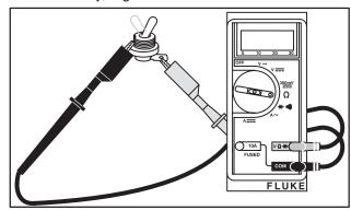
Fig. 108 – CHECKING TOGGLE STOP SWITCH
