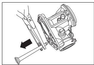
Fig. 150 – REMOVING PICK-UP TUBE VACU-JET CARBURETOR
