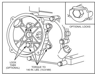
Fig. 134 - INSTALLING GEAR CASE
