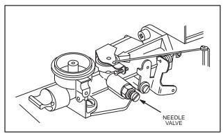
Fig. 140 - CARBURETOR ADJUSTMENT
