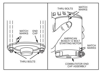
Fig. 684 - REMOVING THRU BOLTS
