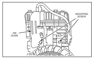
Fig. 101 – INSTALLING IGNITION ARMATURE AND AIR GUIDE
