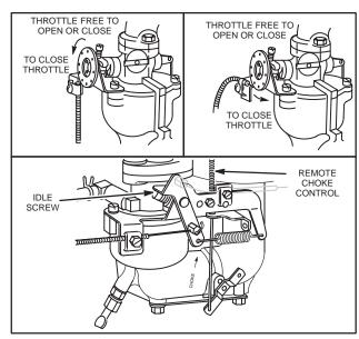
Fig. 354 - REMOTE THROTTLE CONTROL
