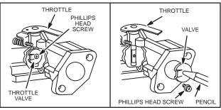
Fig. 131 - REMOVING AND INSTALLING **NEW STYLE THROTTLES**
