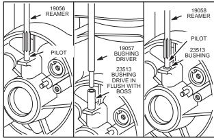
Fig. 93 – INSTALLING BREAKER POINT BUSHING
