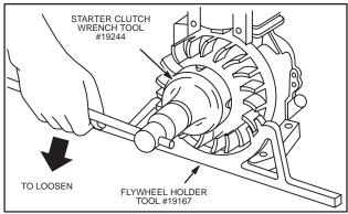
Fig. 79 – REMOVING REWIND STARTER CLUTCH
