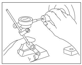
Fig. 150 – CHECKING END PLAY WITH DIAL INDICATOR
