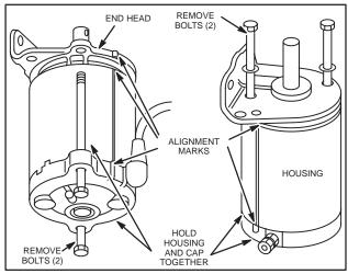
Fig. 699 - REMOVING THRU BOLTS
