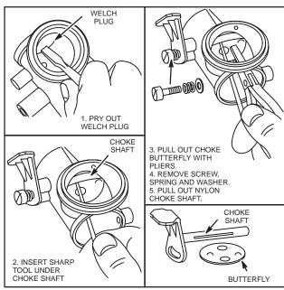
Fig. 274 - NYLON CHOKE SHAFT
