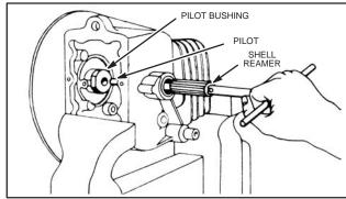
Fig. 909 – REAMING MAGNETO BEARING (SHELL REAMER)
