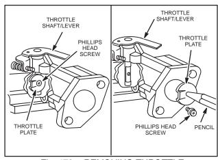
Fig. 178 - REMOVING THROTTLE
