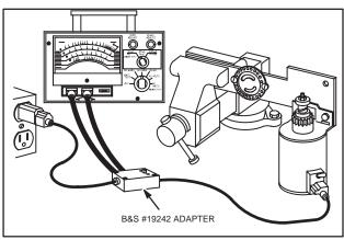
Fig. 683 – TESTING 120 VOLT STARTER MOTOR **VOA METER**
