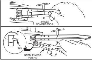
Fig. 511 - REMOVING SPRING
