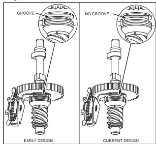
Fig. 156 - CAM GEAR AND CLUTCH
