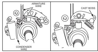
Fig. 87 – INSTALLING STYLE II BREAKER POINTS
