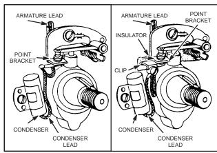
Fig. 35 - REPLACING CONDENSER
