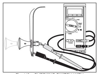
Fig. 112 – CHECKING SWITCH WITH PLASTIC KEY
