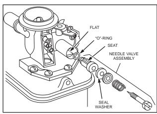
Fig. 168 – NEEDLE VALVE ASSEMBLY PRESS-IN TYPE
