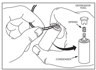
Fig. 90 – REMOVING OR INSTALLING WIRES ON CONDENSER
