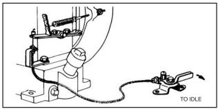
Fig. 364 – MODELS B, ZZ REMOTE THROTTLE CONTROL
