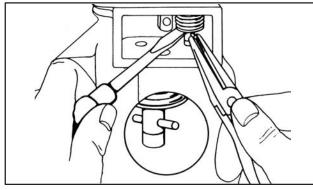
Fig. 498 – REMOVING VALVES AND REPLACING VALVES
