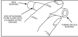
Fig. 62 – INSTALLING BUSHING AND PLUNGER
