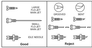
Fig. 262 - MIXTURE NEEDLES
