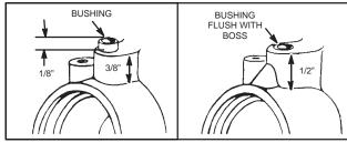
Fig. 20 – INSTALLING BREAKER POINT BUSHING
