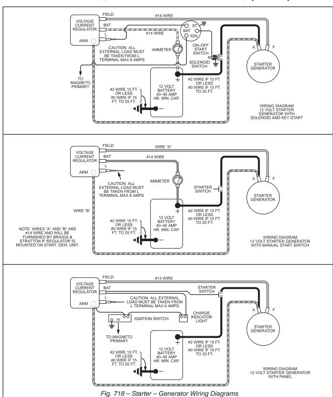
Starter-Generator Wiring Diagram
