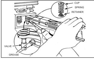
Fig. 507 - REMOVING VALVES
