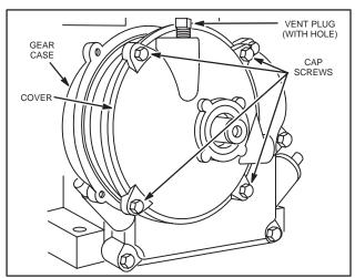
Fig. 130 – DRAINING GEAR REDUCTION AND REMOVING COVER
