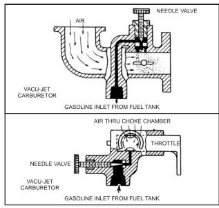
Fig. 125 - VACU-JET CARBURETORS
