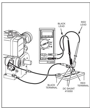
Fig. 783 – TESTING REGULATOR-RECTIFIER 16 AMP SYSTEM WITH DC SHUNT
