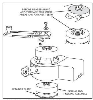
Fig. 639 – INSPECTING PARTS & REPLACING SPRING CUP
