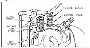
Fig. 495 - ADJUSTING VALVES
