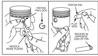
Fig. 540 - REMOVING ROD
