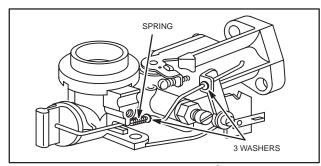
Fig. 201 - CHOKE-A-MATIC® LINKAGE
