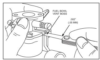
Fig. 270 – CHECKING CARBURETOR BODY
