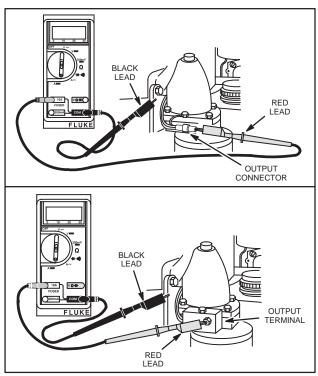
Fig. 740 - CHECKING ALTERNATOR OUTPUT
