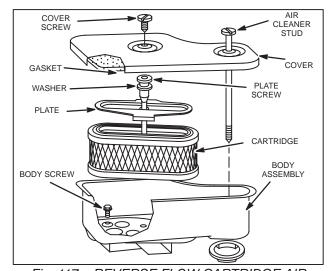
Fig. 117 – REVERSE FLOW CARTRIDGE AIR CLEANER, VERTICAL CRANKSHAFT
