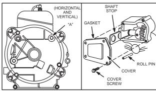
Fig. 345 - SEALANT ON SCREW "A"
