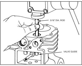
Fig. 527 – PRESSING VALVE GUIDE DOWN
