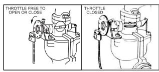
Fig. 377 – MODELS I, N, 5, 6, 8 REMOTE THROTTLE CONTROL
