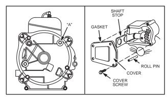
Fig. 340 - SEALANT ON SCREW "A"
