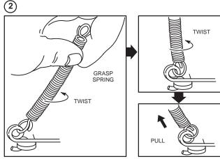
Fig. 332 – REMOVE SPRING FROM EYELET IN LINK
