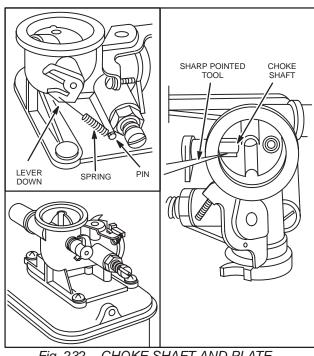
Fig. 232 – CHOKE SHAFT AND PLATE – CHOKE-A-MATIC®
