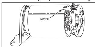
Fig. 714 - ASSEMBLING STARTER
