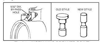
Fig. 21 – INSTALLING BREAKER POINT BUSHING
