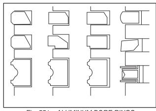
Fig. 551 - ALUMINUM BORE RINGS
