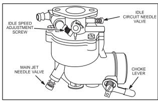
Fig. 267 – MEDIUM FLO-JET, HORIZONTAL CRANKSHAFT
