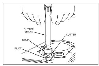
Fig. 521 - COUNTERBORING FOR VALVE SEAT
