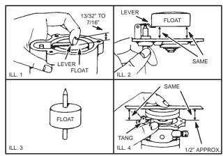
Fig. 278 - CHECKING FLOAT POSITION (EARLY)
