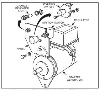
Fig. 715 - STARTER PANEL ASSEMBLY
