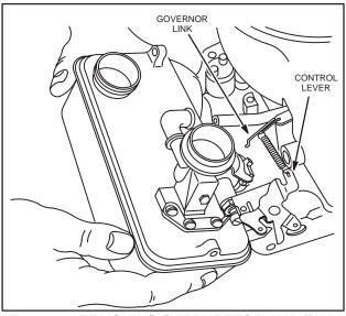
Fig. 143 – REMOVING CARBURETOR AND TANK ASSEMBLY
