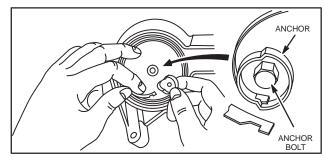
Fig. 619 - REMOVING SPRING ANCHOR
