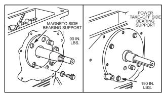
Fig. 890 - INSTALLING BEARING SUPPORTS
