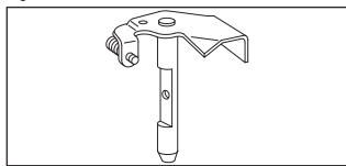
Fig. 228 – THROTTLE SHAFT AND LEVER
