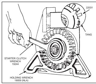
Fig. 12 - ASSEMBLING FLYWHEEL
