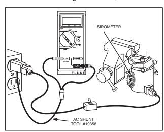
Fig. 668 – TESTING 120 VOLT STARTER MOTOR – DIGITAL MULTIMETER
