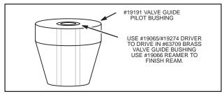
Fig. 516 - MODIFIED PILOT TOOL #19191
