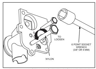
Fig. 236 – INSTALLING FUEL PICK-UP TUBE
