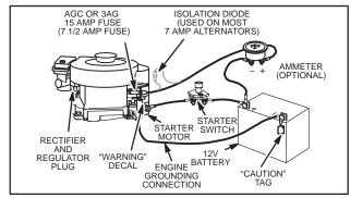
Fig. 751 - TYPICAL WIRING INSTALLATION
