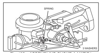
Fig. 185 – ASSEMBLING CHOKE-A-MATIC® LINKAGE
