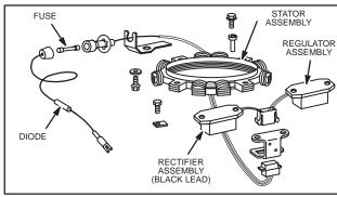
Fig. 750 - 7 AMP ALTERNATOR ASSEMBLY
