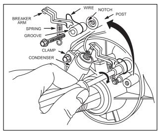
Fig. 95 – INSTALLING STYLE II BREAKER POINTS
