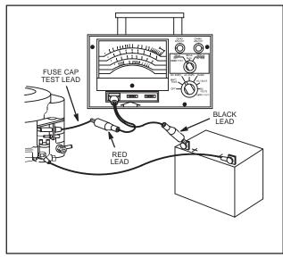
Fig. 753 – TESTING ALTERNATOR OUTPUT
