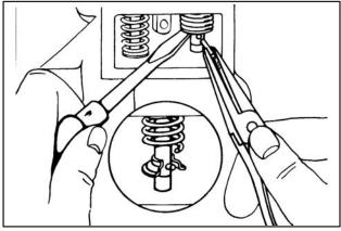
Fig. 502 - REMOVING VALVES AND REPLACING **VALVES**
