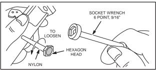
Fig. 179 – REPLACING NYLON FUEL PICK-UP TUBE
