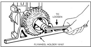
Fig. 10 – REMOVING FLYWHEEL NUT (1/2" DIA. THREADS)
