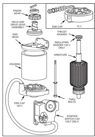
Fig. 698 - 12 VOLT & 120 VOLT STARTER MOTOR - EXPLODED VIEW
