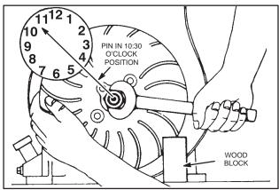
Fig. 13 - ASSEMBLING FLYWHEEL
