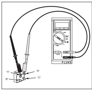
Fig. 705 - TESTING RECTIFIER
