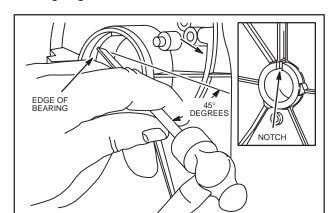
Fig. 922 – NOTCHING CYLINDER OR CRANKCASE COVER
