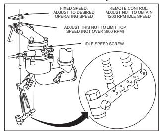
Fig. 329 - ADJUSTING TOP LOAD RPM
