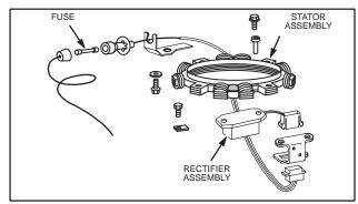
Fig. 746 - ALTERNATOR ASSEMBLY
