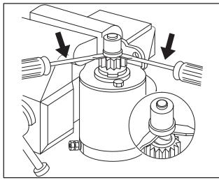
Fig. 693 - REMOVING CAP ASSEMBLY (SOME MODELS)
