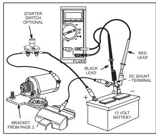
Fig. 696 – TESTING 12 VOLT STARTER MOTOR
