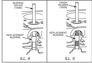
Fig. 515 - BUSHING VALVE GUIDES
