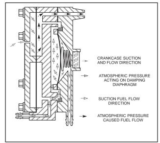
Fig. 312 – FUEL FLOW CRANKCASE VACUUM, TYPICAL
