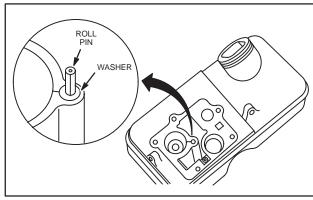
Fig. 235 – INSTALLING ROLL PIN AND TEFLON WASHER
