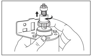
Fig. 678 - CHECKING STARTER MOTOR DRIVE
