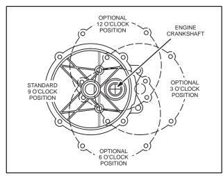
Fig. 140 – POSITIONING GEAR CASE ASSEMBLY
