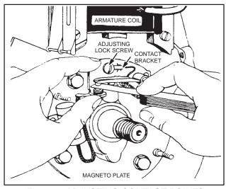
Fig. 34 - ADJUSTING CONTACT POINTS
