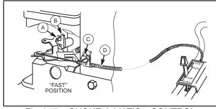
Fig. 217 – CHOKE-A-MATIC® CONTROL, TYPICAL
