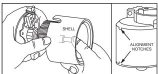
Fig. 659 - INSERTING ARMATURE
