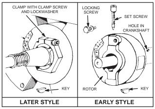
Fig. 43 - REMOVING ROTOR
