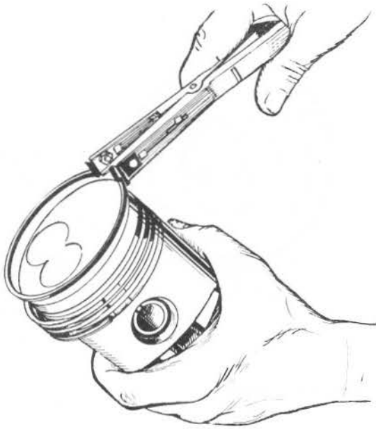
FIGURE 30. REMOVING PISTON RINGS
