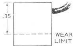
FIGURE 21. BRUSH WEAR LIMIT
