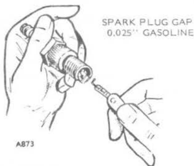
FIGURE 14. SPARK PLUG GAP
