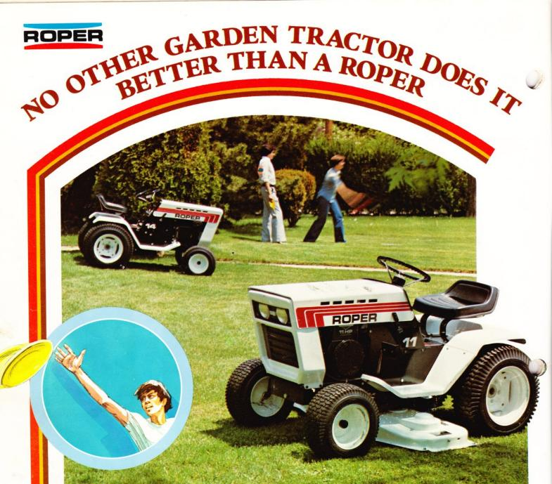
Power mowing is fun, fast and easy with a Roper 11 HP Model T1228BR (lower right). Ruggedly built with a fourcycle Briggs & Stratton Synchro-balanced engine. It has powerful guts to finish the chores. Features include Roper 6 + 2 Pac all-gear transmission with 6 speeds forward, 2 speeds in reverse.
