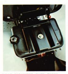
REAR MOUNTED FUEL TANK (selected models) Affords easier, safer filling, eliminates spillage on hot engines. Seat tilts forward for quick access to tank. Fuel pump assures proper fuel-flow to engine.
