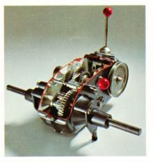
ROPER 6 + 2 PAC POWER TRAIN Rugged Roper-built all-gear transmission provides 6 precise speeds forward from .85 to 6.56 mph, plus 2 reverse speeds of 1.02 and 2.53 mph.
