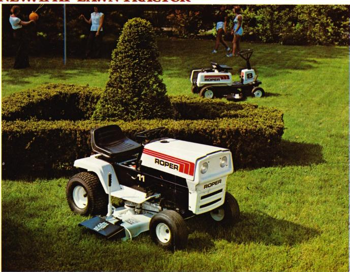
Powered by 11 HP Briggs & Stratton Syncro-balanced engine. Handles easily, maneuvers quickly. Standard equipment: PTO assembly, four speeds (3 forward and 1 reverse), key start, adjustable tie rods, automotive type steering, low tone muffler, full fenders, foot rests, 36" cut, and spring seat.
