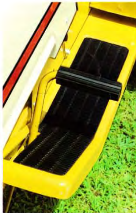
Rubber tread on foot rest provides good footing for the tractor operator against grass and loose dirt.
