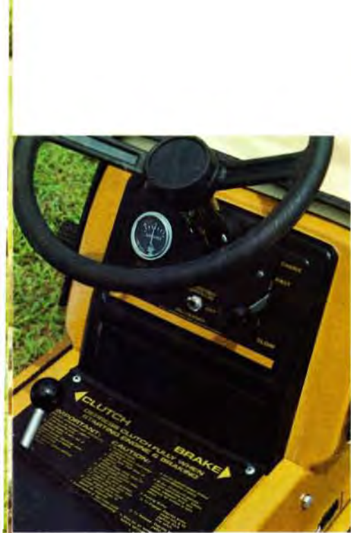
Dashboard area includes controls such as ammeter, electric start key-lock switch and throttle-choke—all grouped for easy control and accessibility. You'll find safety and operating instructions located there, too.
