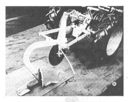
The 3-point hitch makes the adaptability of the "Suburban" tractor complete. It is shown here, with all linkage in place, and with the plow properly mounted to it. This 3-point hitch makes the application of the various tools to the tractor quite simple.
