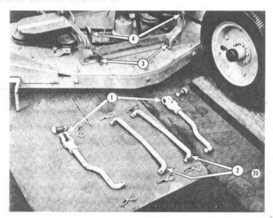
In order to give clearance for mounting the mower, as shown, drive front wheels of the tractor up on 2 x 4 blocks to raise tractor height. Lock the rear brakes. Remove adjusting brackets (No. 1) and lower parallel links (No. 2) from mower. Now slide the mower under the tractor from the right side, until the center mandrel is directly beneath the center of the tractor frame.
