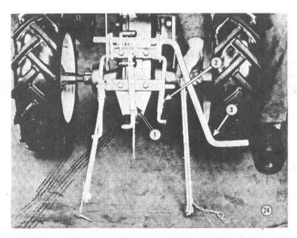
The two adjusting mechanisms on the three point hitch can easily be seen.
