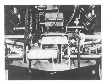
This head-on view of the tractor shows the mower, jackshaft and belts in place. In order to hook up the center drive belt, place the mower clutch lever in the extreme rear position (disengaged). Bring the center drive belt over the tie rod, through the front axle bracket and install on the inner drive sheave (No. 1) of the jackshaft. From this front position the belt should be twisted so that the left hand side goes to the top of the
