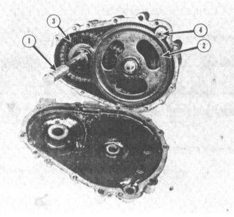
This is the interior of the transmission with the transmission cover removed, showing axle and gear (No. 1), plus the intermediate shaft and gear (No. 2). These must be removed together as the triple strand roller chain (No. 3) holds them as a single unit. The input shaft is No. 4.
