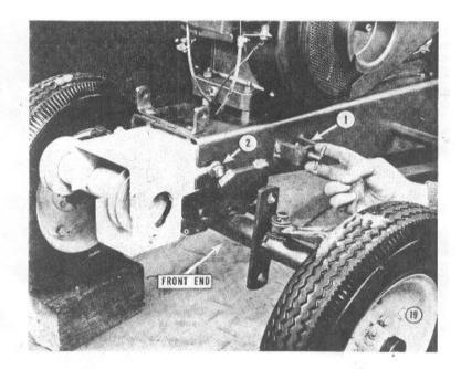
To mount the jackshaft shown, for mower operation, pull plungers (No. 1) on both left and right side of the tractor frame to allow the jackshaft frame to lock into tractor frame. Pull the jackshaft frame forward in order to
