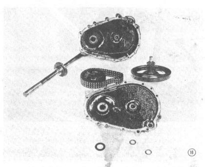
Illustrated are all working parts removed from the transmission case,
