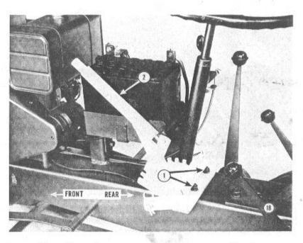
Here the rotary mower lift lever assembly is shown bolted to the tractor frame. The rear bolts (No. 1) of the frame are mounted in the steering column plate. The lift lever (No. 2) is on the left side of the tractor. Each notch changes the height of cut of the mower approximately 3/8".
