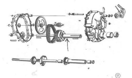
This is an exploded view of the transmission.
