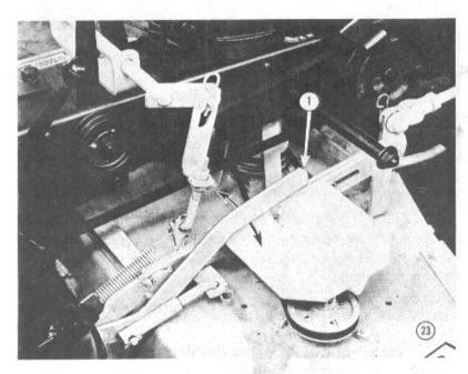
The mower clutch lever (No. 1) is shown in the engaged position. With the clutch lever in this position the center drive belt will be tight. Adjust the belt guides shown in the previous picture on
